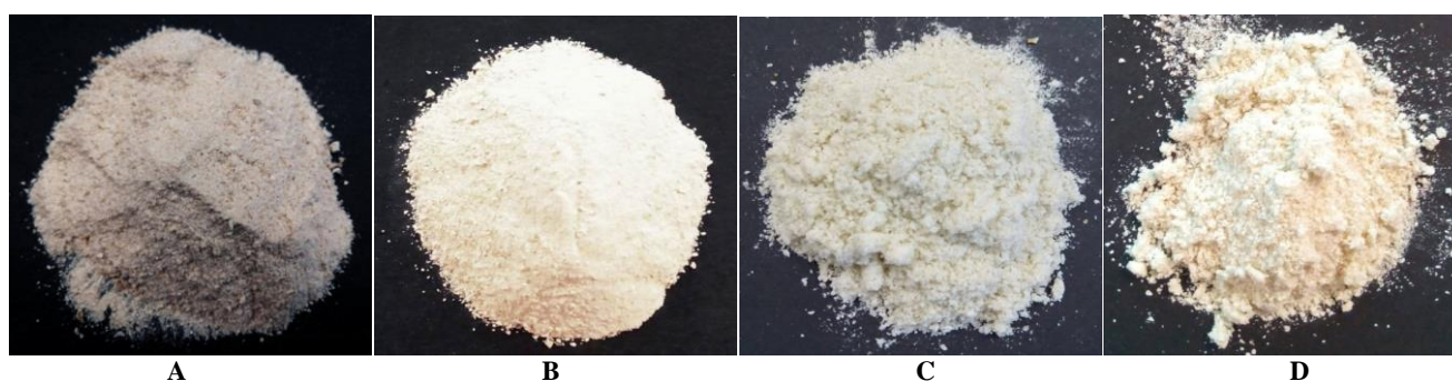
Figure 1. A. Sardinella fimbriata fish bone powder before drying in the oven; B. S. fimbriata fish bone powder after drying in the oven; C. Clarias gariepinus bone powder before drying in the oven; D. C. gariepinus bone powder after drying in the oven
