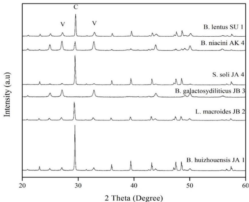
**Figure 3.** The result of XRD analysis for identified CaCO<sub>3</sub> crystal forms. (C stands for calcite peak, the highest peak occurs in 29°2θ, V: stands for vaterite peak, the highest peak occurs in 27°2θ and 32°2θ).
