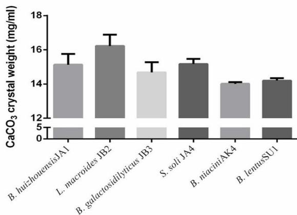
**Figure 2.** The weight of CaCO<sub>3</sub> crystals precipitated by carbonatogenic bacteria
