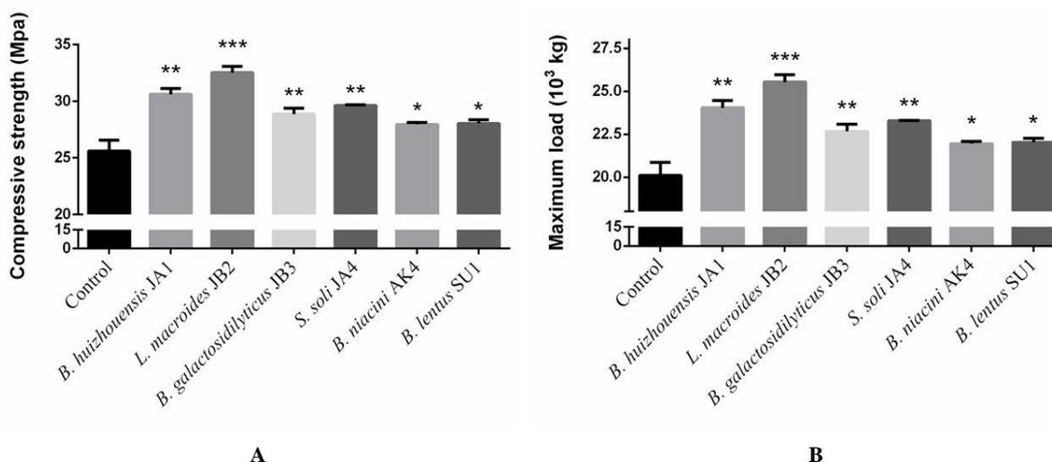
**Figure 6.** The compressive strength and maximum load of control concrete and bio concrete with the carbonatogenic bacterial application
