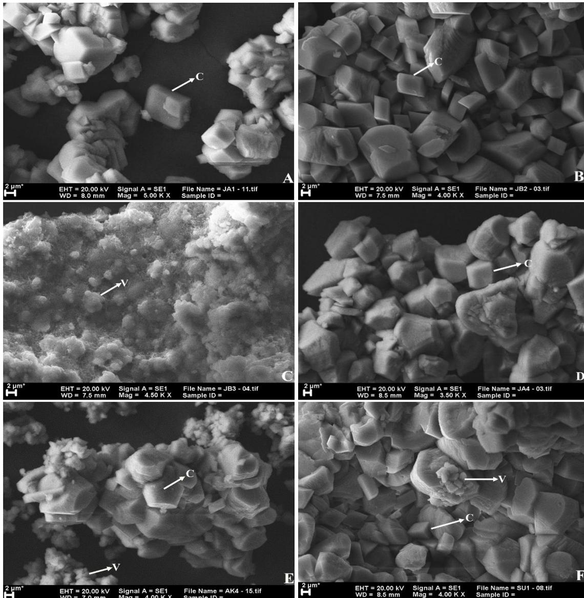
**Figure 4.** The shape of the  $\text{CaCO}_3$  crystal was revealed by the SEM micrograph. A. *B. huizhouensis* JA1 formed rhombohedral crystal; B. *L. macroides* JB2 formed rhombohedral crystal; C. *B. galactosidilyticus* JB3 formed hexagonal crystal; D. *S. soli* JA4 formed rhombohedral crystal; E. *B. niacini* AK4 formed rhombohedral and hexagonal crystal and F. *B. lentus* SU1 formed rhombohedral and hexagonal crystal (C stands for calcite, V stands for vaterite)
