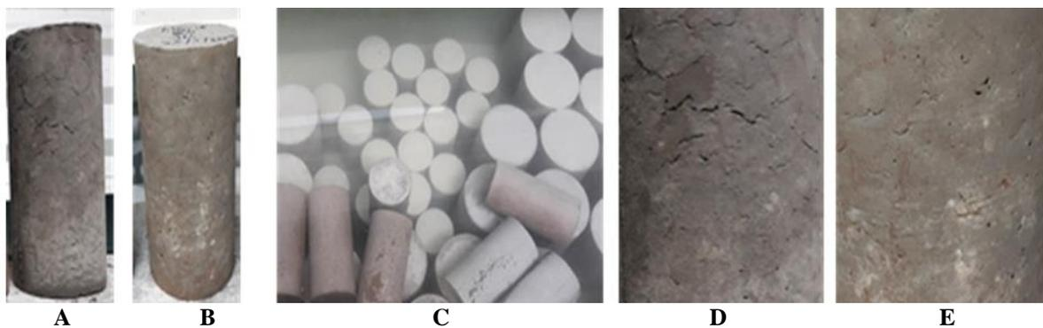
**Figure 5.** Morphology of concrete. A. Control concrete (without carbonatogenic bacterial application); B. Bio concrete with carbonatogenic bacterial application; C. Curing process of concrete specimens; D. Surface morphology of control concrete; E. Surface morphology of bio concrete with carbonatogenic bacteria application
