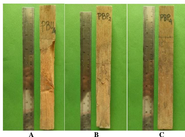
**Figure 8.** Damage caused by termites to the samples of *Styrax sumatrana* wood from Pakpak Bharat: A. Heavy, B. Moderate, C. Light
