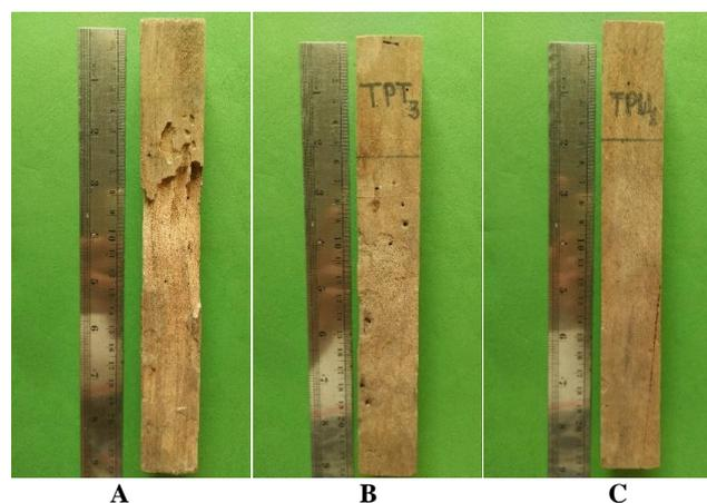
**Figure 9.** Damage caused by termites to the samples of *Styrax sumatrana* wood from North Tapanuli: A. Heavy, B. Moderate, C. Light
