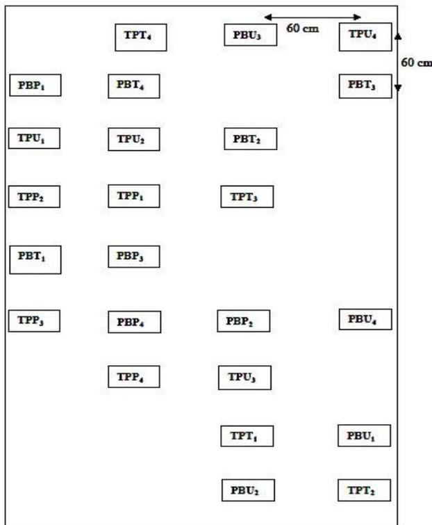
**Figure 2.** The layout of the wood resistance testing using Graveyard Test method
