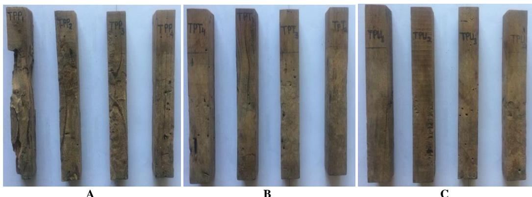
**Figure 6.** The appearance of *Styrax sumatrana* wood from North Tapanuli after 100 days of testing based on the axial positions of the stem: A. Base, B. Middle, C. Top
