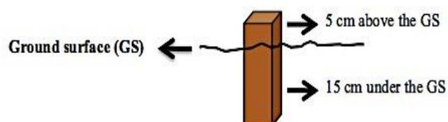
**Figure 1.** Diagram of wood resistance testing using Graveyard Test method by burying the sample under the soil and left the upper part above the soil.
