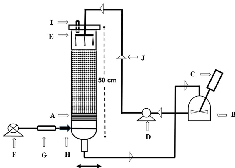
**Figure 1.** Bioleaching column design. A. Plate, B. Bioreactor, C. Stirrer, D. Peristaltic pump, E. Liquid distributor, F. Air compressor, G. Air filter, H. Air inlet, I. Gas outlet, J. Connector
