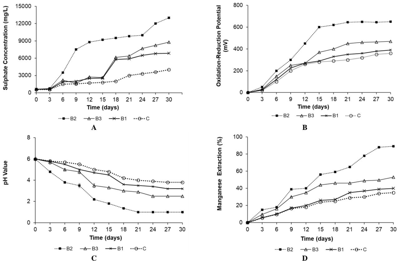
**Figure 2.** Changes in sulfate concentration (A), ORP (B), pH (C), and manganese extraction (D) during column bioleaching by a mixed culture of indigenous bacteria with biochar addition. Note: B: Biochar addition, B1: 0.2%; B2: 0.4%; B3: 0.6%. C: without biochar addition
