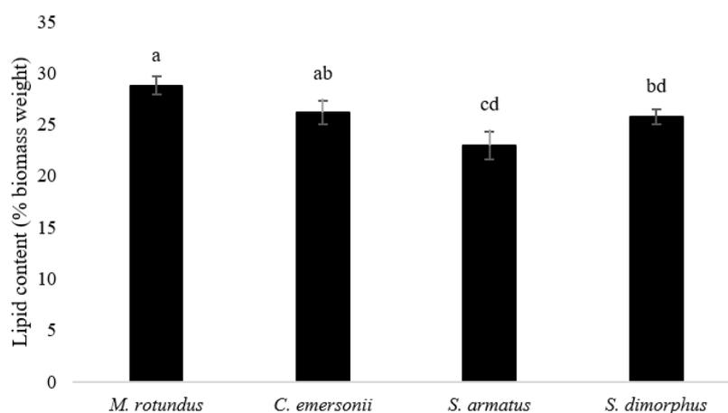
**Figure 6.** Microalgae lipid contents extracted by Bligh Dyer method. The superscript letter above the bar lipid content showed the significant value by ANOVA analyses with Bonferroni post hoc test at significance 0.05
