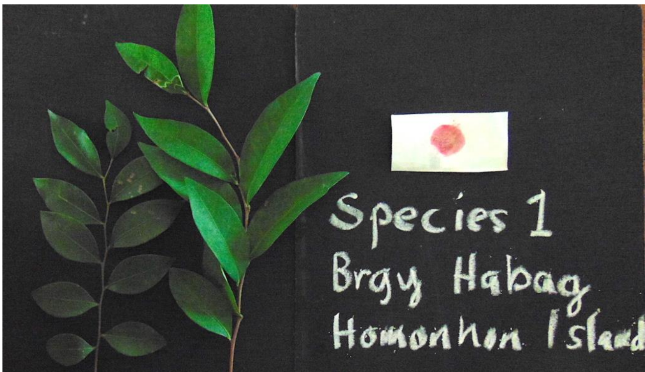
Figure 3. Phyllanthus securinegoides Merr., shown as a nickel hyperaccumulator by a field test using filter paper impregnated with 1% dimethylglyoxime dissolved in 95% ethanol. Photograph by R.B. Romero and I.A. Navarrete
