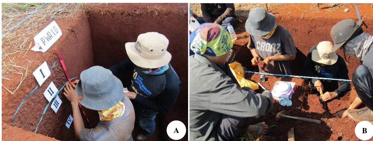
Figure 3. Soil survey activities: (A) Determining horizon in every profile for identifying the diversity of soil layer; (B) Collecting soil sample for laboratory analysis.
