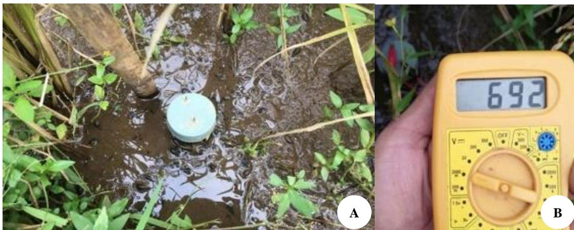
**Figure 2.** A. MFC prototype in the rice field, B. Measurement of electric Voltage on MFC using the multiparameter tool
