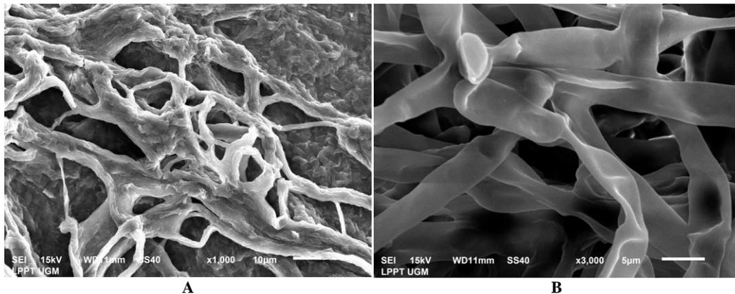
**Figure 3.** Scanning electron micrographs of mycelia of *Colletotrichum scovillei* treated with *Paenibacillus polymyxa* C1 (A) and control (B)**Table 5.** Compounds detected in cell-free filtrate of *Paenibacillus polymyxa* C1
