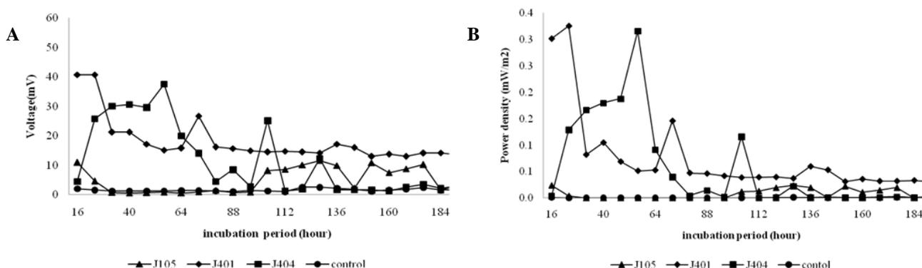
Figure 6. The voltage output as a function of time from the MFC with rice straw (0.3% w/v) as a substrate and catalyzed by different cellulose-degrading bacteria (A), power density (B) also as a function of time from the MFC
