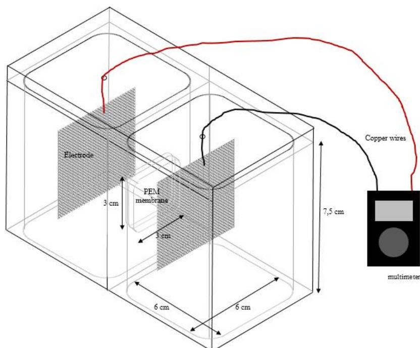
**Figure 1.** Schematic picture of MFC system
