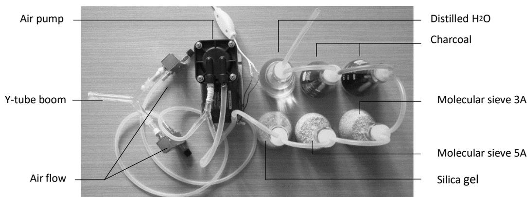
**Figure 1.** Experimental unit for the olfactory response test
