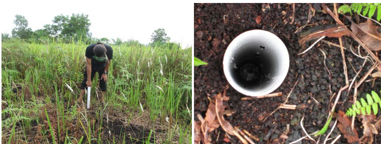
Figure 3. Piezometer measurement and set up in a peatland site impacted by an overflow dam
