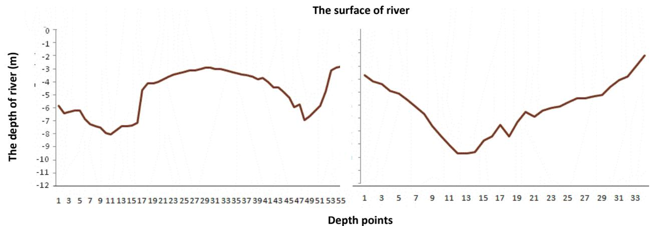
Figure 4. Base topography of Mahakam River, East Kalimantan, Indonesia. The left is the estuary of Sungai Payau (a tributary of the Mahakam) with width of 0.28 km; the right is Sungai Payau with width of only 0.20 km
